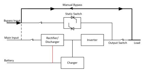
Fig .2-5 Maintenance mode operation diagram
