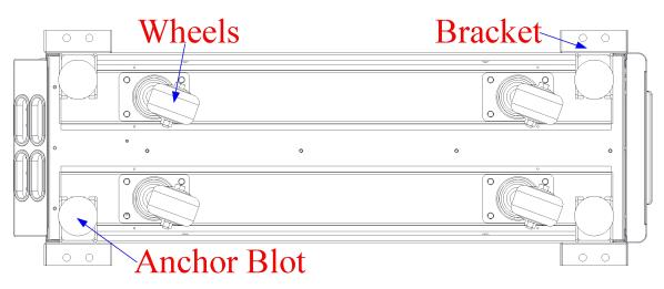
Fig.3-1 Supporting structure (Bottom view)
