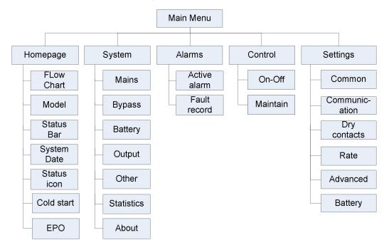
The menu structure of the monitoring display interface is shown in Fig. 4-2.
