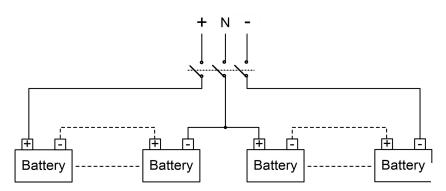
Fig 3-2 Battery string wiring diagram
