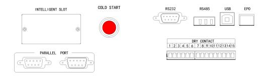
Fig.3-6 Dry contact & communication interface
