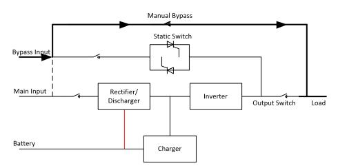
Fig. 2-4 Bypass mode operation diagram
