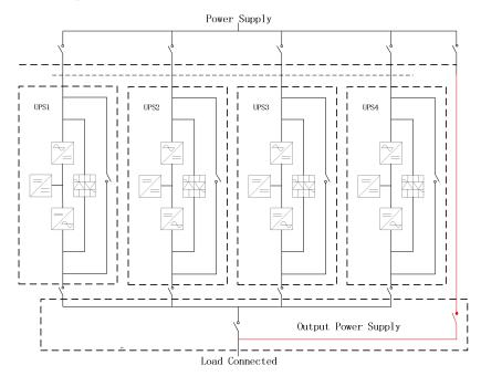
Fig. 5-5 Parallel diagram
