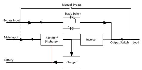
Fig 2-3 Battery mode operation diagram
