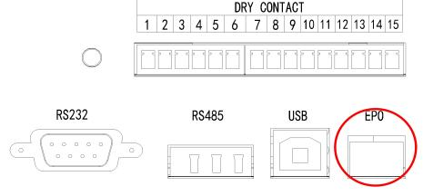
Fig. 5-5 EPO port in communication interface
