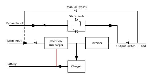
Fig.2-6 ECO Mode operation diagram
