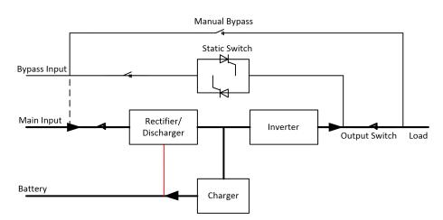
Fig 2-2 Normal mode operation diagram
