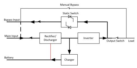
Fig.2-7 self aging operation diagram
