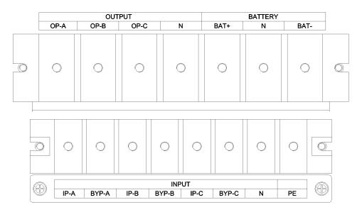
Fig.3-5 connections terminals for 40-60kVA model
