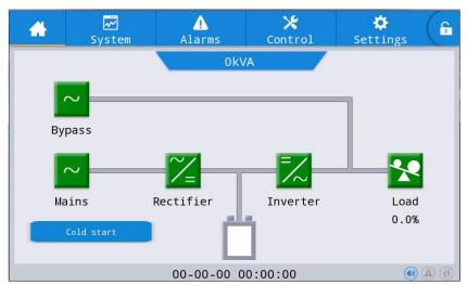
Fig. 5-1 The cold start button in LCD
