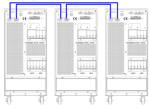
Fig.5-6 Parallel connection
